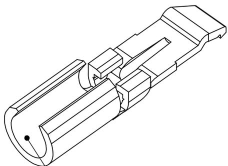
BARREL SIZED FOR #16-20 AWG WIRE
