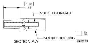
1. HOUSING AND CONTACT ASSEMBLIES ARE UL RECOGNIZED PER E2226 AND CSA CERTIFIED PER LR251 54.
