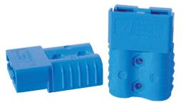
Like the other Multipole connectors, the SB<sup>°</sup> 120 offers colorcoded mechanically keyed housings. Keys can be used to identify and separate different circuits, or prevent users from accidentally cross mating different voltages. Wires sizes from 10 to 1 AWG (5.3 to 42.4 mm<sup>2</sup>) are held in the second smallest SB<sup>°</sup> housing.
