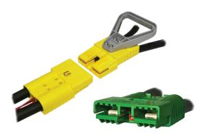
SBE<sup>®</sup> and SBX<sup>®</sup> connectors can integrate up to 8 auxiliary power/ signal contacts along with the two primary power circuits. Sequencing within auxiliary positions is possible using the 4 pin lengths available in the 1x4 auxiliary connector. SBE<sup>®</sup> and SBX<sup>®</sup> offer touch safe housings.
