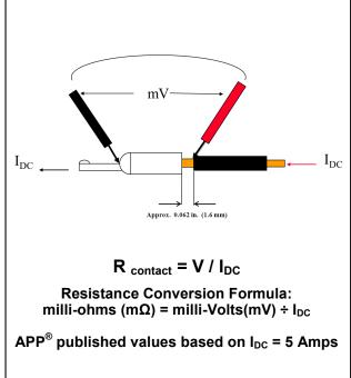
The included crimp performance and dimensional information are provided as a means to verify quality crimping of Anderson Power Products® contacts and is based on the use of tooling. The assembly of connector solutions with tooling assures that all crimp performance and fit specifications are met. Customers must regularly re-check electrical performance and dimensions of crimps to determine if crimp tools require maintenance due to wear over time.
